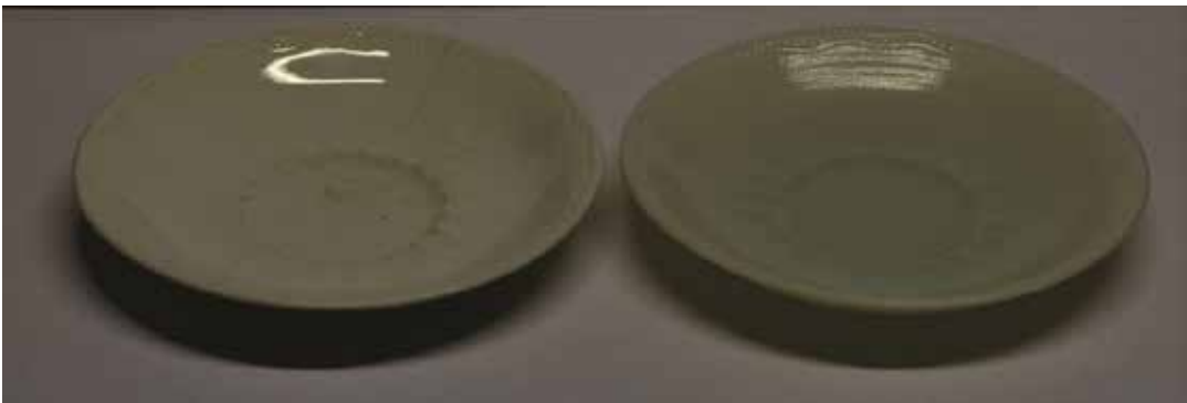
Figure 10: Comparison of details focusing on the surface structure of the original ceramic saucer (right) and the printed physical model (left). With the naked eye, one can see the quality of the physical model compared to the original, especially in terms of details of texture and size
