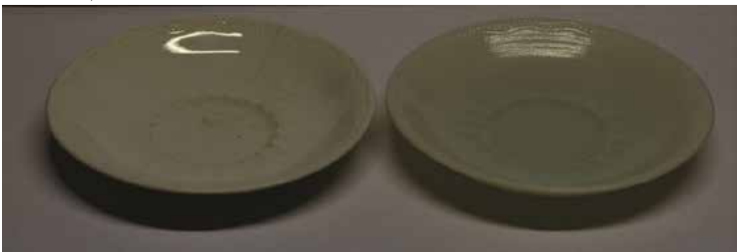
Figure 10: Comparison of details focusing on the surface structure of the original ceramic saucer (right) and the printed physical model (left). With the naked eye, one can see the quality of the physical model compared to the original, especially in terms of details of texture and size
