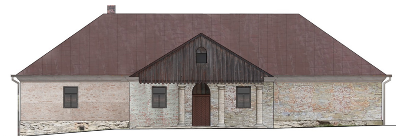
Fig. 23: Architectural and structural survey of the manor building. Front, south-facing elevation with the colour, texture and material types shown. By M. Krupa, D. Kuśnierz-Krupa, Ł. Bednarz, 2021.
