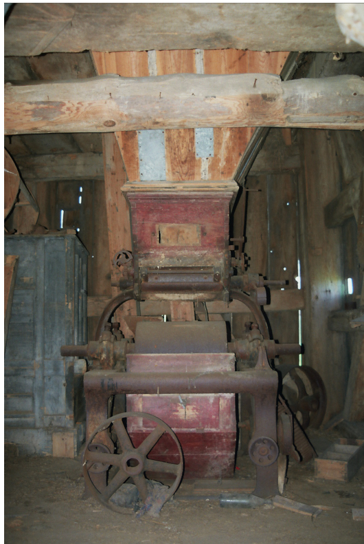
Fig. 19: A roller mill inside the windmill from Zawada (before translocation); photo by F. Tomaszewski, 1999.
