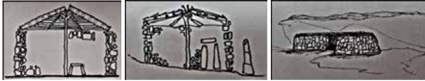
Fig. 10: Top: Gombe and its section Bottom: Types of Gombes; use of natural materials without industrial processing. 37
